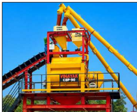
WEIGHING & BATCHING SYSTEM
